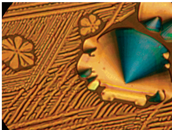
FIGURE 5. Texture of the discotic mesophase (Col ho ) of 1b at 183.3 °C obtained by cooling from the isotropic liquid.
